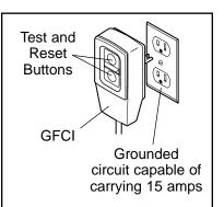
USING THE CONTROLS on page 12). Once the unit is running, press the GFCI "test" button. The spa should shut off. Press the "reset" button. The spa should resume normal operation. If the spa continues to run after the "test" button is pressed, the GFCI is damaged.
